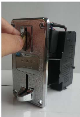
3rd step: drop coin 30 times until LED off 4th step: normal operation
