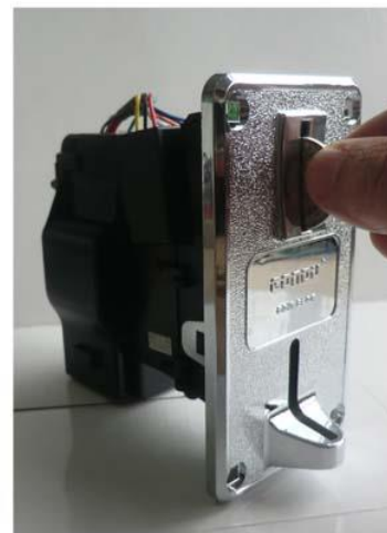
3rd step: drop coin 30 times until LED off 4th step: normal operation
