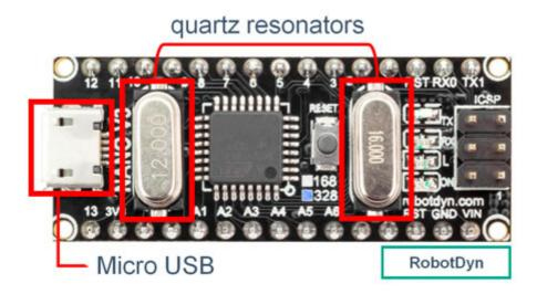
Quartz resonators are more reliable, stable and accurate in comparison with small ceramic ones.
