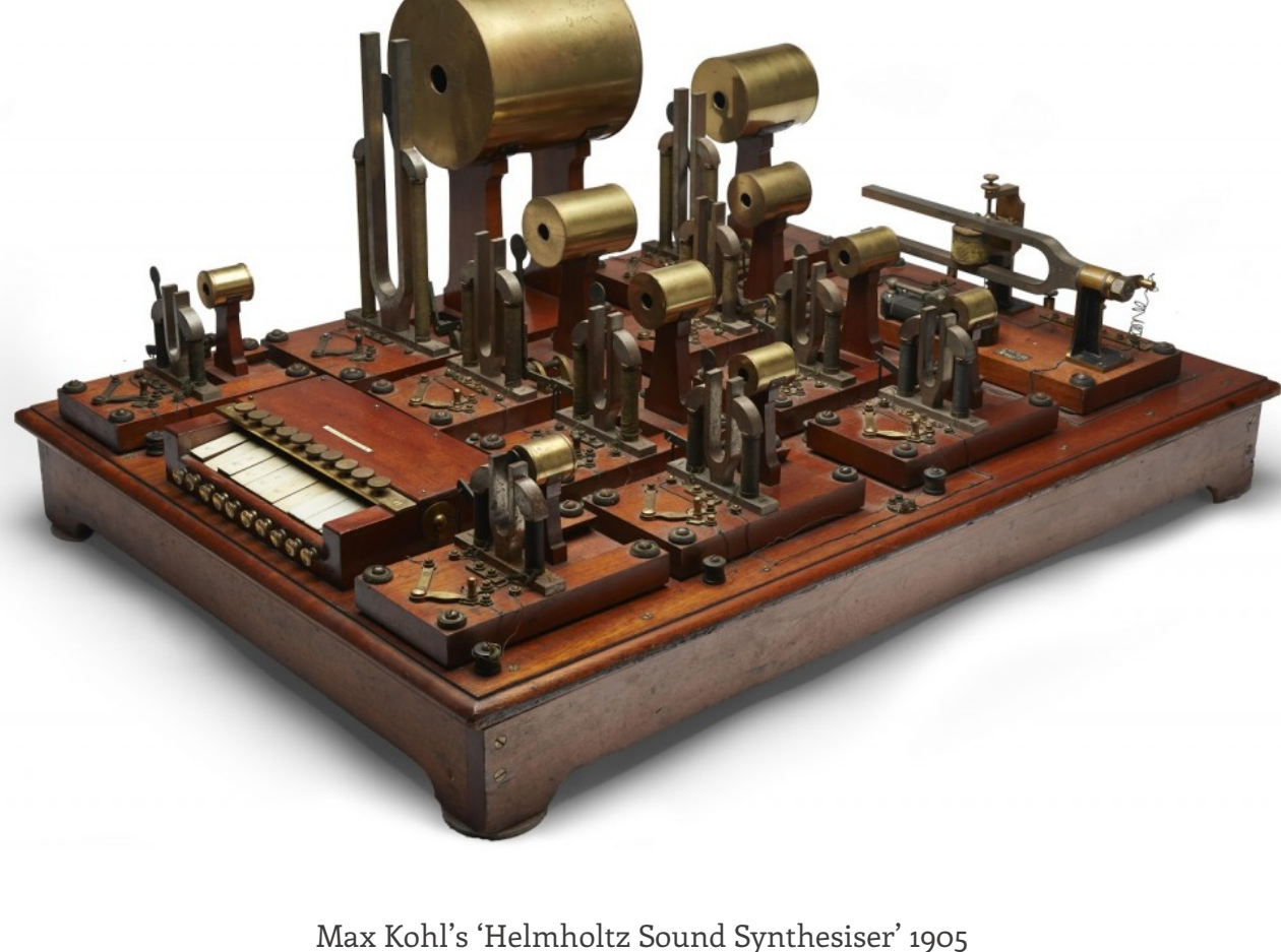
Max Kohl's 'Helmholtz Sound Synthesiser' 1905
