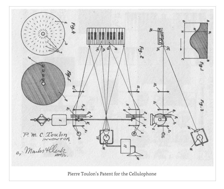
Invented by the French engineer Pierre Toulon aided by the electronic engineer Krugg Bass, the Cellulophone ("Cellule Photo-électrique") made it's debut as a prototype in France in 1927. The Cellulophone was an electro-optical tone generator instrument resembling an electronic organ controlled by two eight octave keyboards and a foot pedal board.
