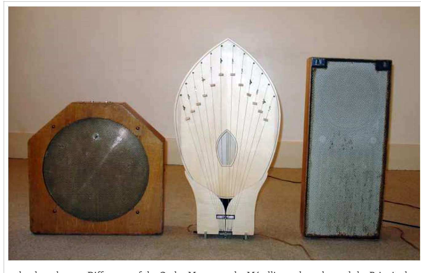
loudspeakers or Diffuseurs of the Ondes Martenot: the Métallique, the palm and the Principal
